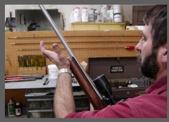
This can be easily tested by gently rapping on the bottom of the forend and listening for the sound of the forend striking the barrel. Hopefully it won't.
