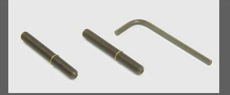
There are two double ended screws that are used to attach the pillars to the action. One end is <sup>1</sup>⁄<sub>4</sub> X 32 and it screws into the action. The other end is <sup>1</sup>⁄<sub>4</sub> X 28, has a hex key recess and screws into the "T" handles.
