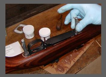
It is also very important that the "T" handles are not over tightened! It is very easy to induce stress in the assembly by over tightening. Once you feel the trigger guard come into contact with the pillars stop and back off the "T" handles just a tiny bit. T.O.C.
