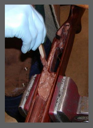
First apply the epoxy compound into the front pillar hole and then completely fill the lug area. The majority of the epoxy should lay flat on the bottom so that when the barreled action is inserted into the stock, the very bottom of the action will come into contact with the epoxy first and the epoxy will then flow up around the receiver eliminating any air bubbles.
