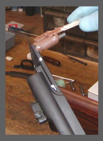
To ensure that there are no air bubbles around the aluminum pillars lay a layer of bedding epoxy around both front and rear pillars.
