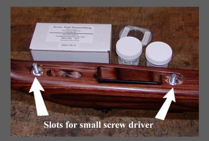
Holding the barrel and action firmly in the stock, use a small screw driver to rotate the adjustment post of each pillar so that it is flush or slightly higher than the level of the stock.
