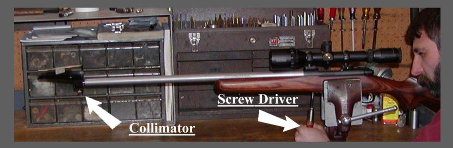
You should not be able to detect any change whatsoever in the collimator's view. Any change in that view illustrates how stresses are changing under the changing load of the guard screws. If there are no stresses there are no changes.
