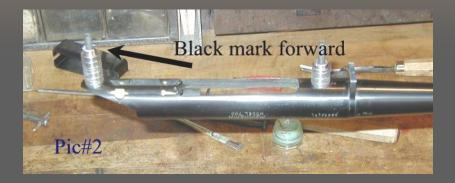
Each pillar has a threaded post with a screw driver slot used for adjusting the pillars length. There is one short pillar used for the front guard screw and one long pillar used at the rear. Each threaded post is cut at 2.5 degrees to match the angle of the trigger guard. You will find a black mark on one of the screw driver slots. This black mark should always be toward the muzzle.
