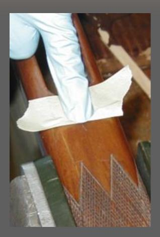
Some bedding epoxies are very runny. To prevent them from running out the bottom of the pillar holes use masking tape to block the bottoms of the holes. This will not be necessary with Pro-Bed 2000
