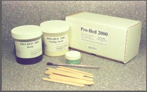
Each *Deluxe Kit* comes with either a black or brown 2 fl oz kit of Pro-Bed 2000 bedding epoxy with release agent. This is a extremely high quality bedding epoxy with a non-critical 1:1 mix ratio by volume. Epoxy mixing instructions are included with the kit.
